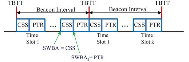
Fig. 11. Synchronized time slots for IEEE 802.11 chipsets.
