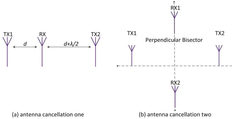
Fig. 3. Antenna cancellation: (a) the scheme in [11]; (b) the scheme in [17].
