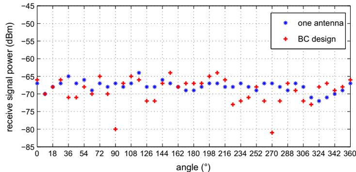
**Fig. 14.** The effect of null positions in the BC design at a distance of 1 m away from the antennas.
