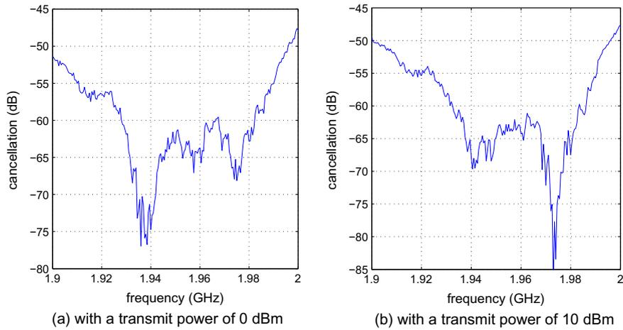
**Fig. 6.** The results of analog cancellation achieved by the BC design: (a) with a transmit power of 0 dBm; (b) with a transmit power of 10 dBm.
