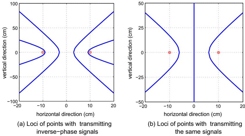
**Fig. 13.** Loci of points where two received signals have inverse phases (the circles indicate the antenna locations): (a) two antennas transmit the same signals; (b) two antennas transmit inverse-phase signals.
