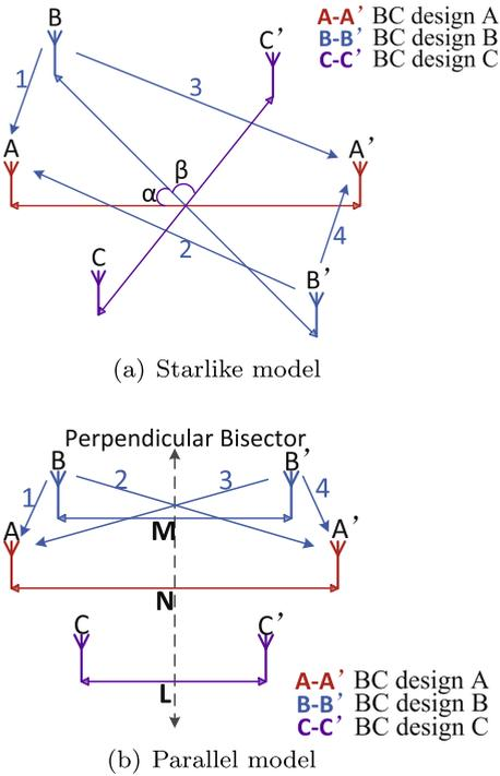
Fig. 4. MIMO extension of the BC design: (a) the starlike model of  $3 \times 3$  MIMO, where the middle points of three BC designs intersect at one point; (b) the parallel model of  $3 \times 3$  MIMO, where the perpendicular bisectors of all the BC designs overlap.
