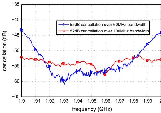
**Fig. 7.** The cancellation results with flat frequency response.
