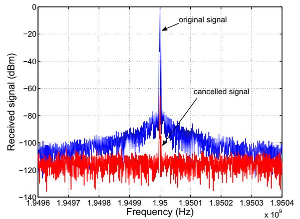
**Fig. 8.** Spectrum leakage of BC design.
