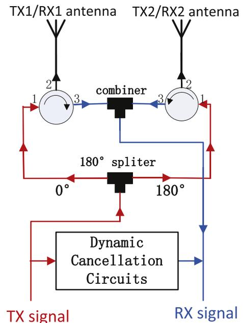
Fig. 2. Integrating the BC design with dynamic cancellation circuits to achieve higher analog cancellation.
