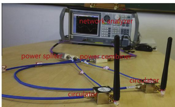
Fig. 5. The implemented BC design and testing equipment.
