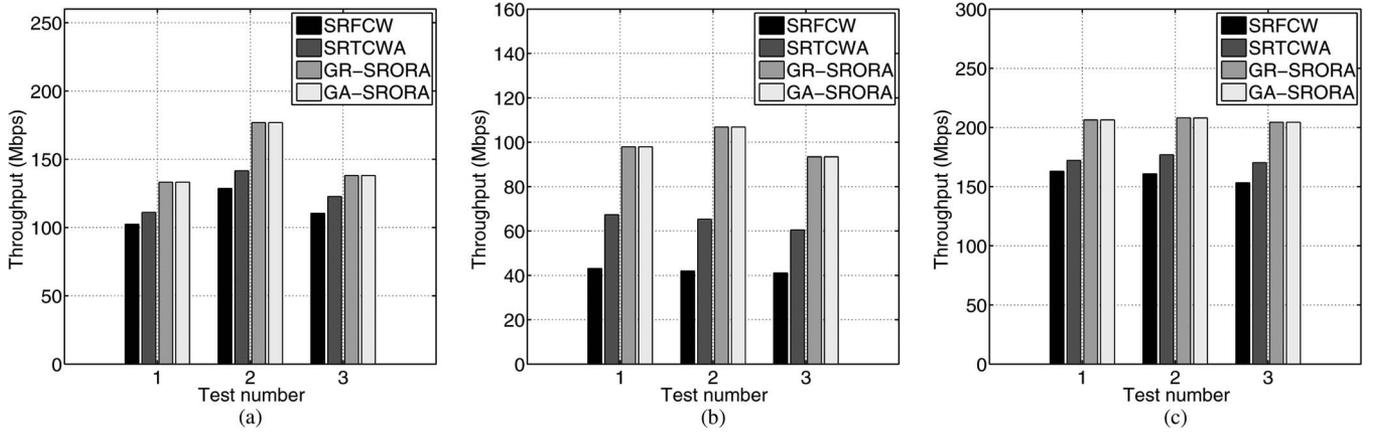
Fig. 7. Network throughput for simple topologies. (a) String topology. (b) Star topology. (c) Grid topology.
