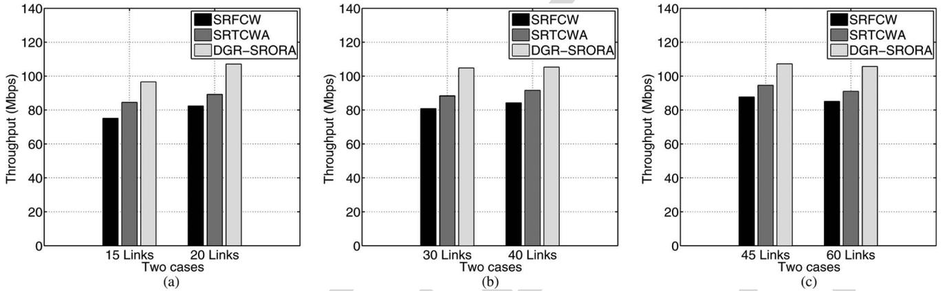
Fig. 8. Network throughput in the scenario of single interference domain. (a) 10 nodes. (b) 20 nodes. (c) 30 nodes.
