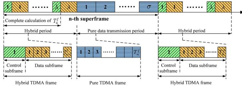
Fig. 3. Frame structure.
