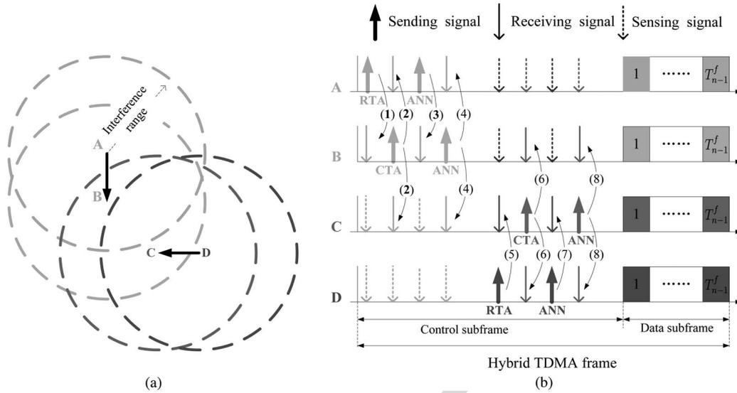
Fig. 4. Operation of the MAC protocol: An example. (a) Topology. (b) Resource negotiation.
