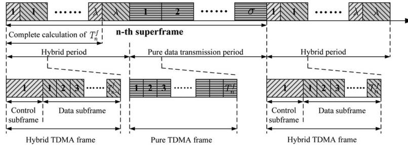
Fig. 3. Frame structure.
