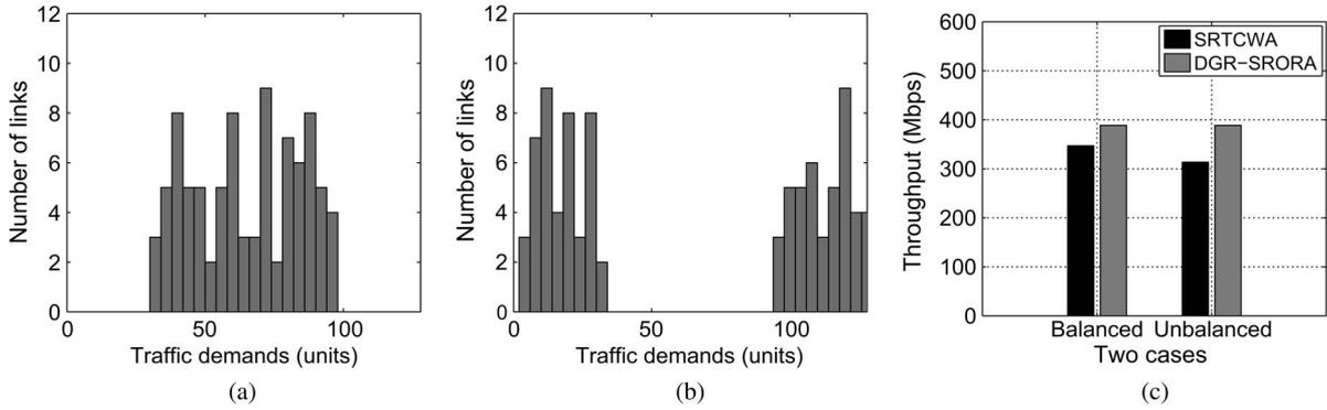
Fig. 10. Network throughput under different traffic distributions. (a) Balanced traffic distribution. (b) Unbalanced traffic distribution. (c) Network throughput.
