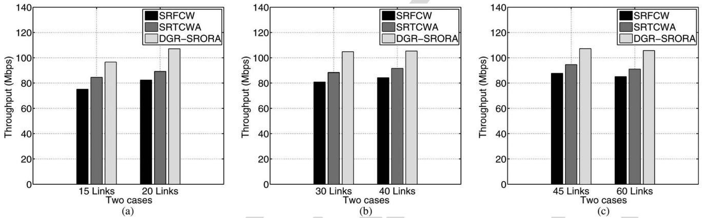
Fig. 8. Network throughput in the scenario of single interference domain. (a) 10 nodes. (b) 20 nodes. (c) 30 nodes.
