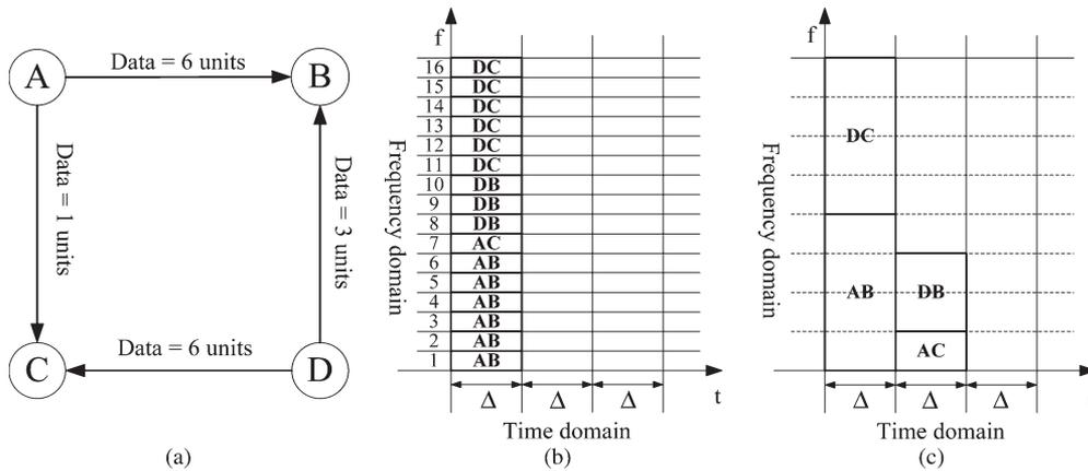
Fig. 1. Benefits of the OFDMA-based channel-width adaptation scheme. (a) Communication topology. (b) OFDMA-based scheme. (c) Traditional scheme.
