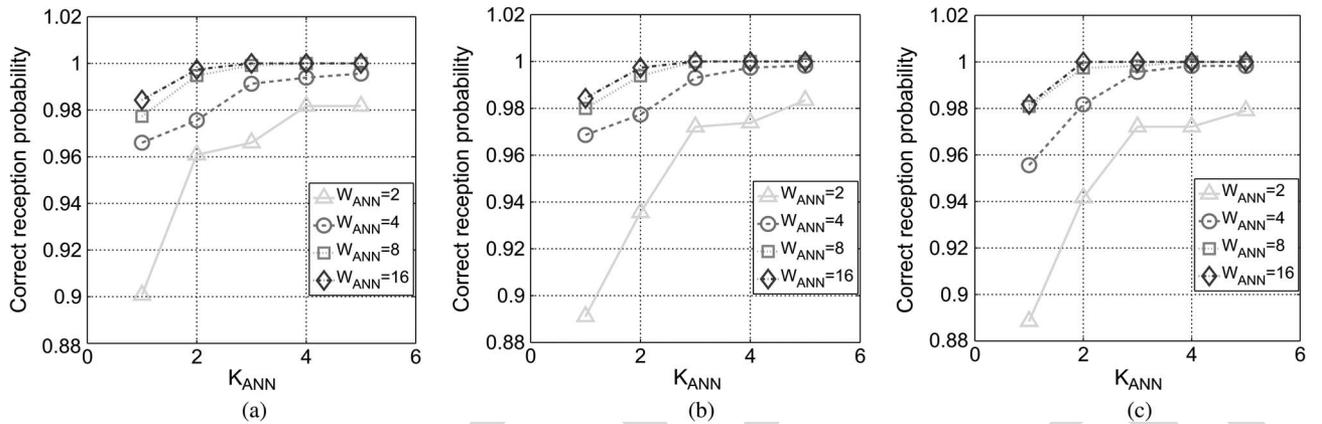
Fig. 11. ANN packet reception probability in the network with multiple interference domains. (a) Control subframe: 10 ms. (b) Control subframe: 15 ms. (c) Control subframe: 20 ms.
